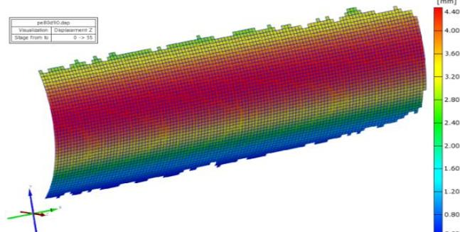
Fig.24. Displacement of the pipe in radial direction (Oz) [mm]
