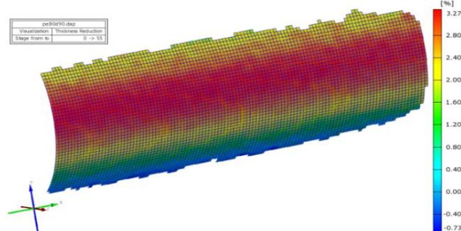
Fig.26. Thickness reduction ( $\delta$ ) [%]
