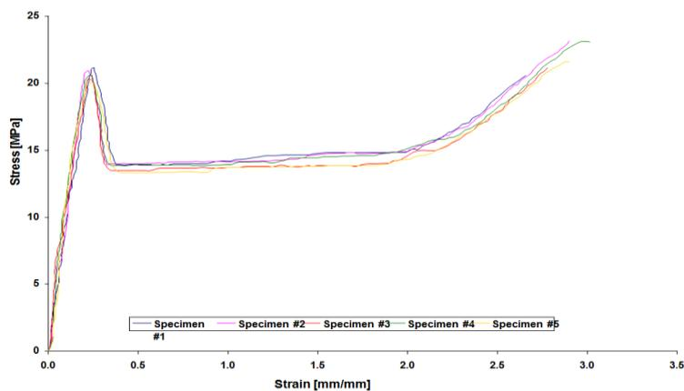
Fig.19. Stress-strain characteristic curves for pipe specimens of  $\Phi$  32 x 3.0 made of PE 100
