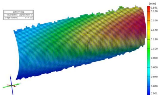
Fig.22. Displacement of the pipe in axial direction (Ox) [mm]
